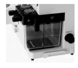
A large 1400ml CO<sub>2</sub> absorber canister features a one-step locking
